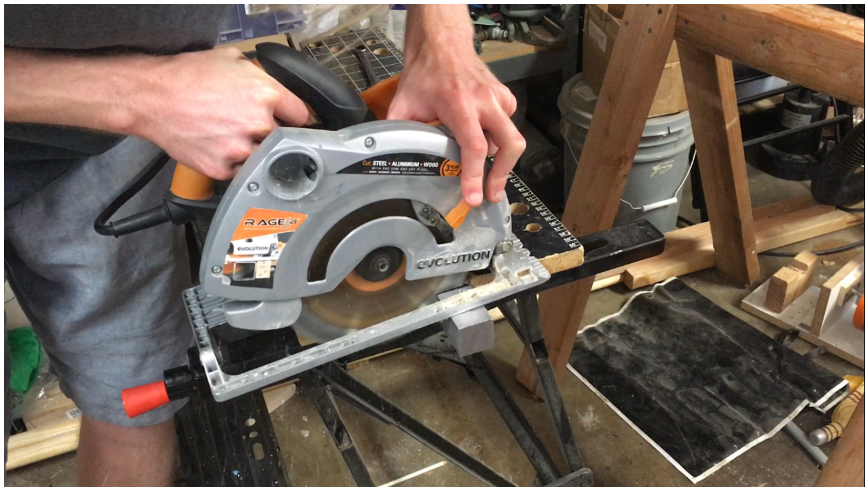
Cutting off a piece of material roughly to size, using a circular saw with a metal cutting blade.
